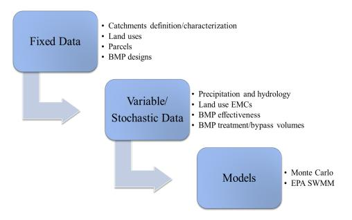
Figure 3. SBPAT Model Data Flow
