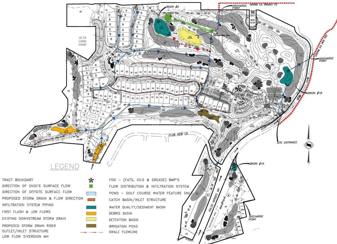
Figure 3-9: Chandler Quarry Project Drainage and Water Quality Concept Plan Source: Hunsaker and Associates. Water Quality Mitigation Plan. June 16, 2010.
