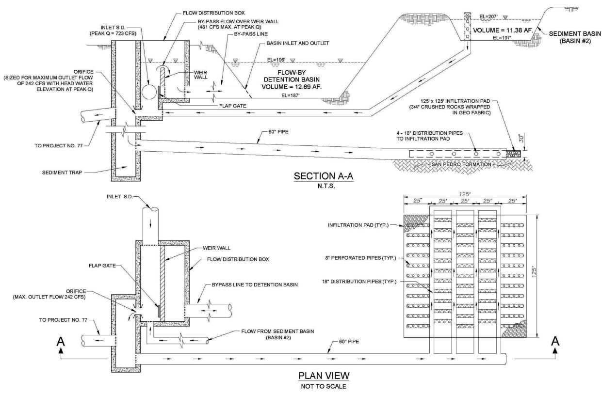
Figure 3-10: Chandler Quarry Project Infiltration System Concept Design Source: Hunsaker and Associates. Water Quality Mitigation Plan. June 16, 2010.
