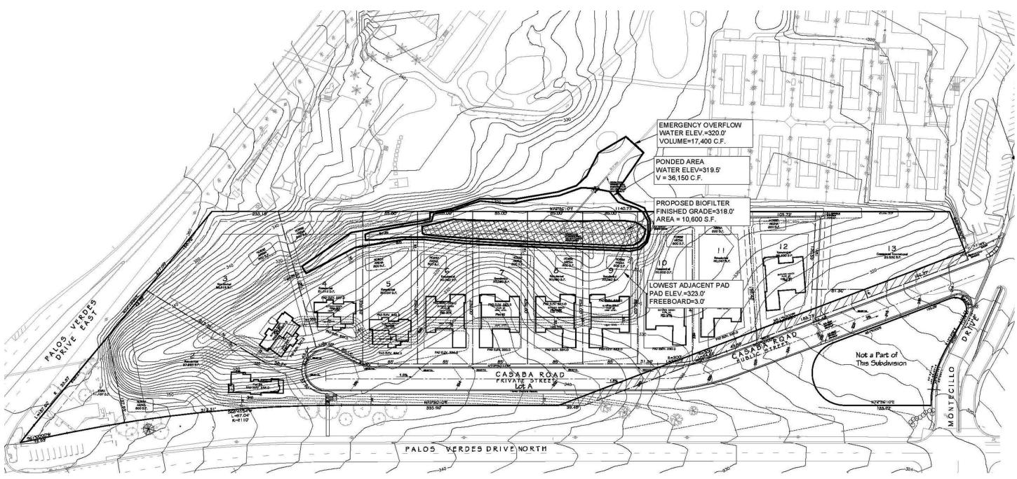
Figure 2: Casaba Estates (formerly Butcher Ranch) Post-Development Design Conditions (Bolton Engineering Corp. Hydrology and Hydraulic Calculations. September 13, 2010).
